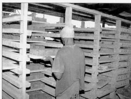
Figure 2 Placing the pallets with the wet bricks on racks for air drying
