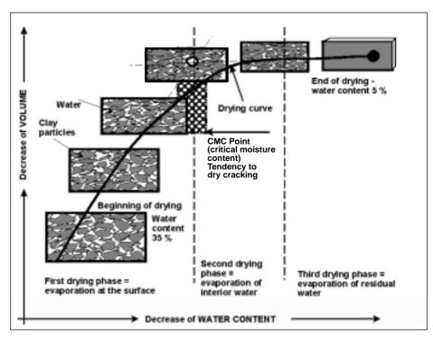
Fig. 2: Schematic drawing of drying in three phases
