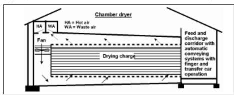
Fig. 10: Schematic drawing of artificial drying: chamber dryer with vertical air flow and with drying charge staying idle
