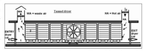
Fig. 11: Schematic drawing of artificial dryer: tunnel dryer with drying charge pushed on dryer cars through horizontal air flow
