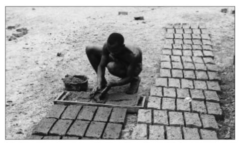
Fig. 4: Correct drying process: green bricks dry slowly in the open in cloudy weather, thus developing no cracks and deformation
