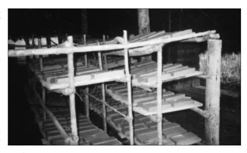
Fig. 6: Simple method of drying floor tiles on racks under a grass roof
