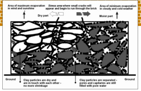
Fig. 3: Schematic drawing of "unbalanced" drying
