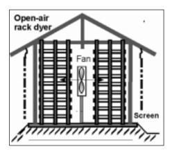
Fig. 9: Schematic drawing of natural drying: rack drying under cover
