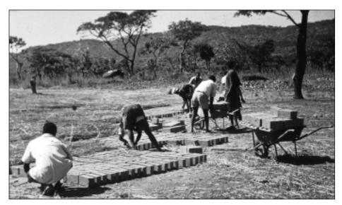
Fig. 7: Bricks are taken by wheelbarrow to the drying ground and turned on edge, covered with grass
